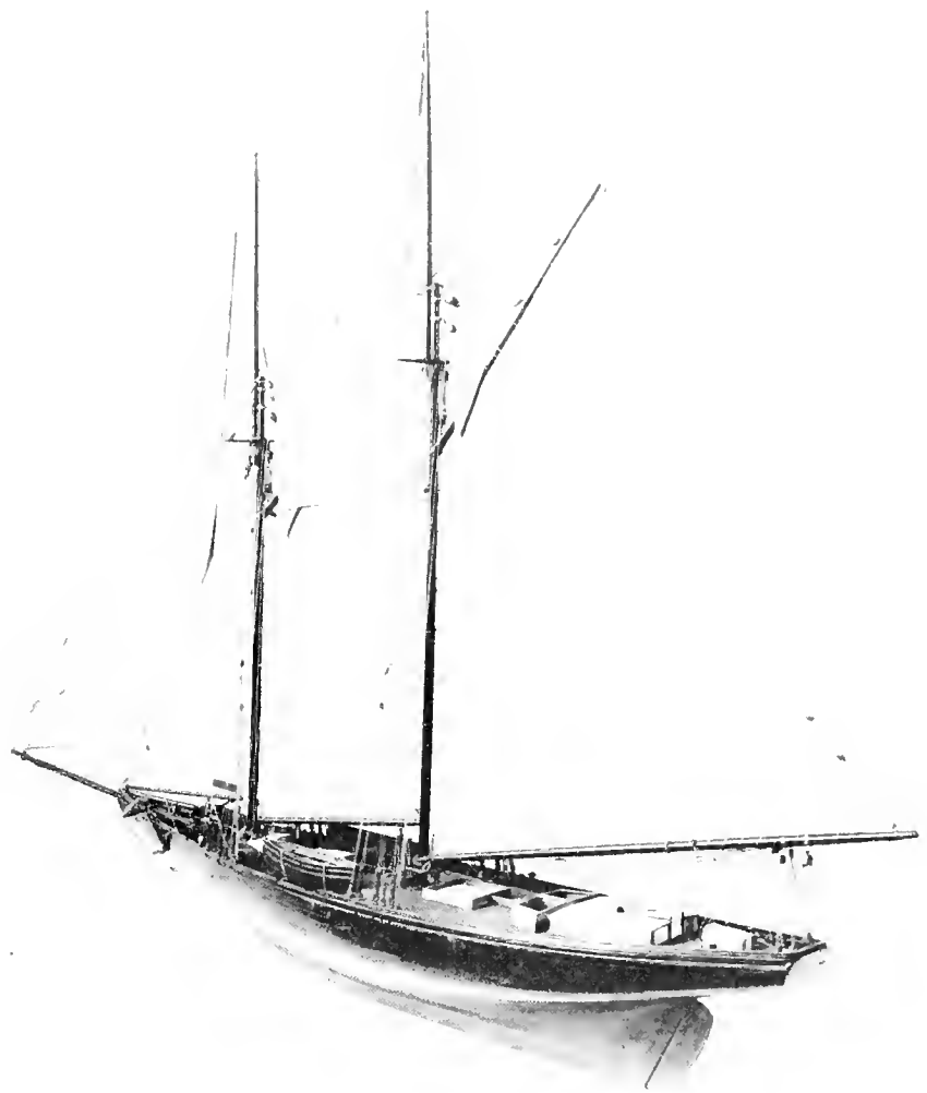
FISHING SCHOONER Rob Roy built at Essex, Massachusetts, in 1900, one of the early fishing schooners designed with a long bow overhang and short keel. For a view afore, see p. 173. Rigged model USNM 298232. (Smithsonian photo 44956.)
